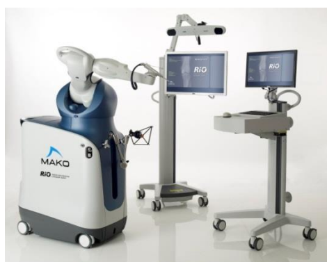
Mako Robotic arm and guiding system
