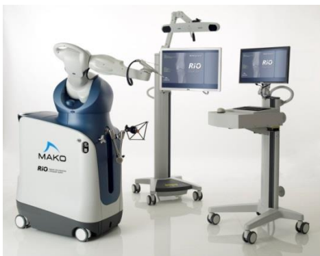
Mako Robotic arm and guiding system
